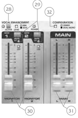
31. MAIN LEFT AND RIGHT FADERS: These are the master left and right faders. If the main outputs are set to dual mono, both have the same signal (sum of left and right) and can be used as zone outputs for house and annex levels etc. These controls are best operated at the 0 (full up) position. It is most important that
